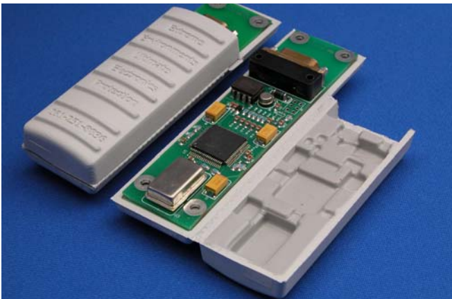
Photo 4: A co-molded Preform
